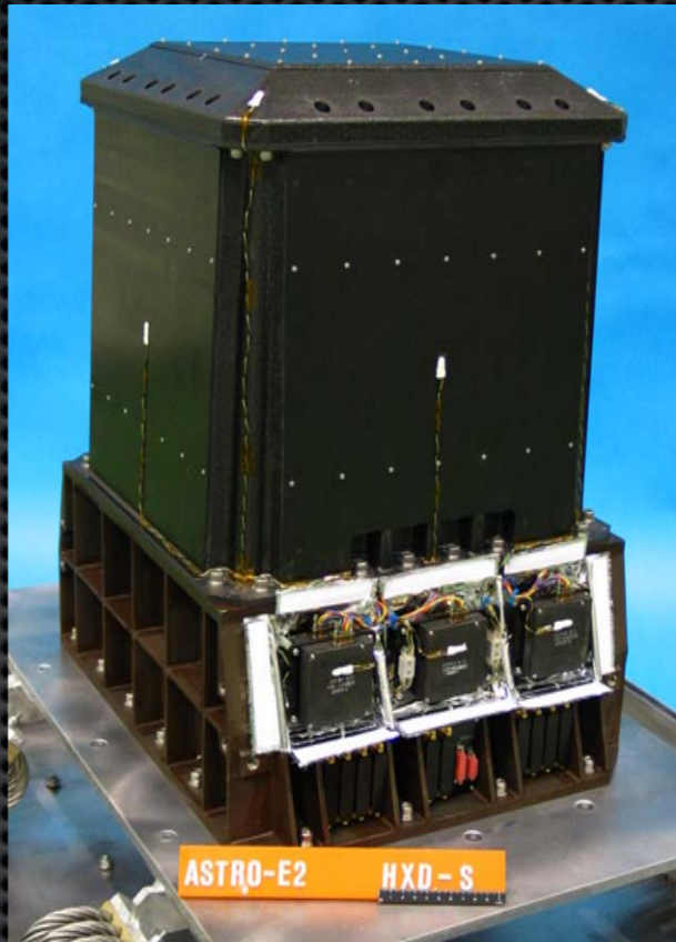
Hard X-ray Detector (HXD) non-imaging spectrometer (10 - 600 keV)
