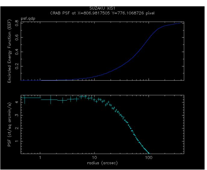
Since the current observation mode is the full-window mode (8-s CCD exposure) and the 0.1-s burst option, the effective exposure is 0.1/8 = 0.0125 times shorter (the actual count rate is 8/0.1 = 80 times higher).
