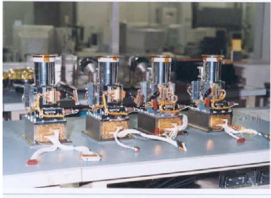
Figure 3.15: (left) The four XIS detectors before installation onto Suzaku . (right) Schematic view of the XIS CCD (top view). The CCD consists of four segments (A, B, C, and D), each with a dedicated read-out node.
