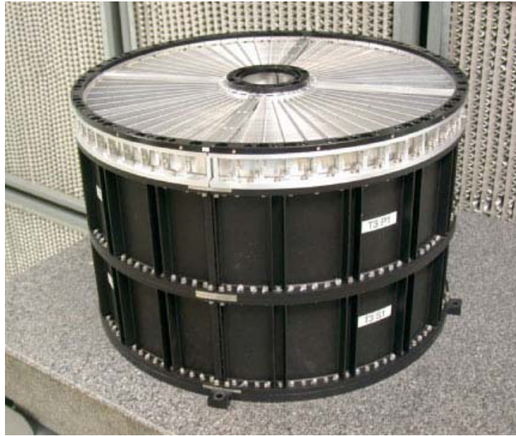
Fig. 3.6: A Suzaku X-Ray Telescope (Serlemitsos et al. 2007).
