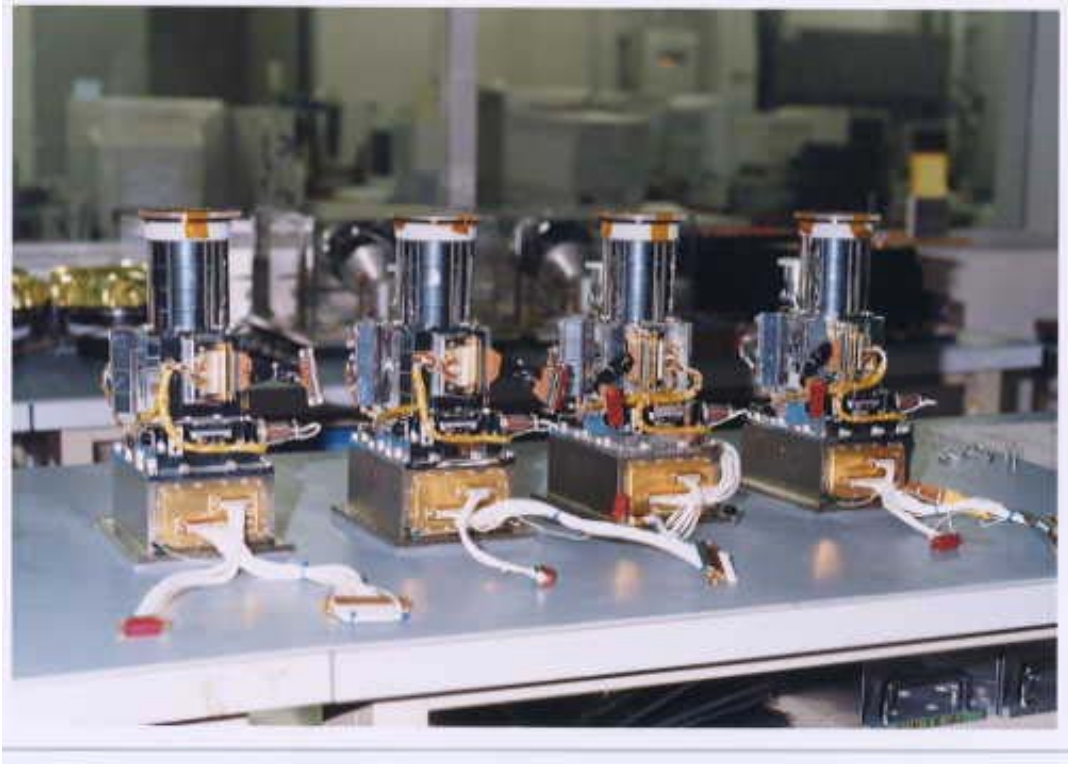
Fig. 3.14: The four XIS detectors before installation onto Suzaku (Koyama et al. 2007).
